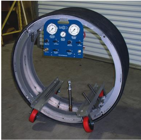
30"-36" Aluminum Collapsible Multi-Size Joint Tester / Grout Packer - Low Pressure
